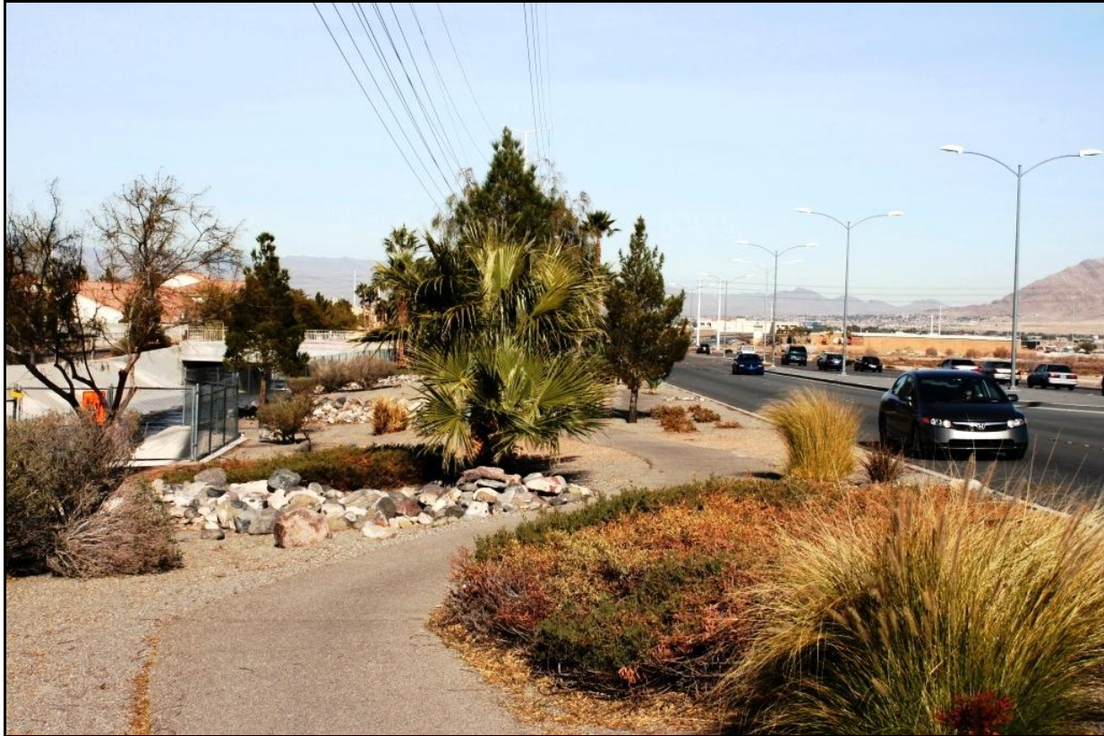
Figure 20: Pedestrian Buffer Between Roadway And Meandering Sidewalk
